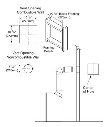
Figure 9 - Vent Opening Requirements
